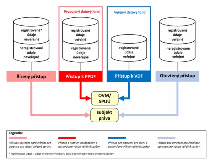
The last figure in this chapter shows the technical way in which remote access to the data (within the meaning of §3(2) of the InfoZ) is ensured. The PPDF and VDF are accessed via a reference interface. Controlled and open access are provided through interfaces exposed to the public internet.
